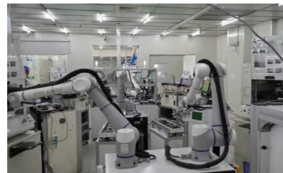
PCB Board Burn-in Transportation
